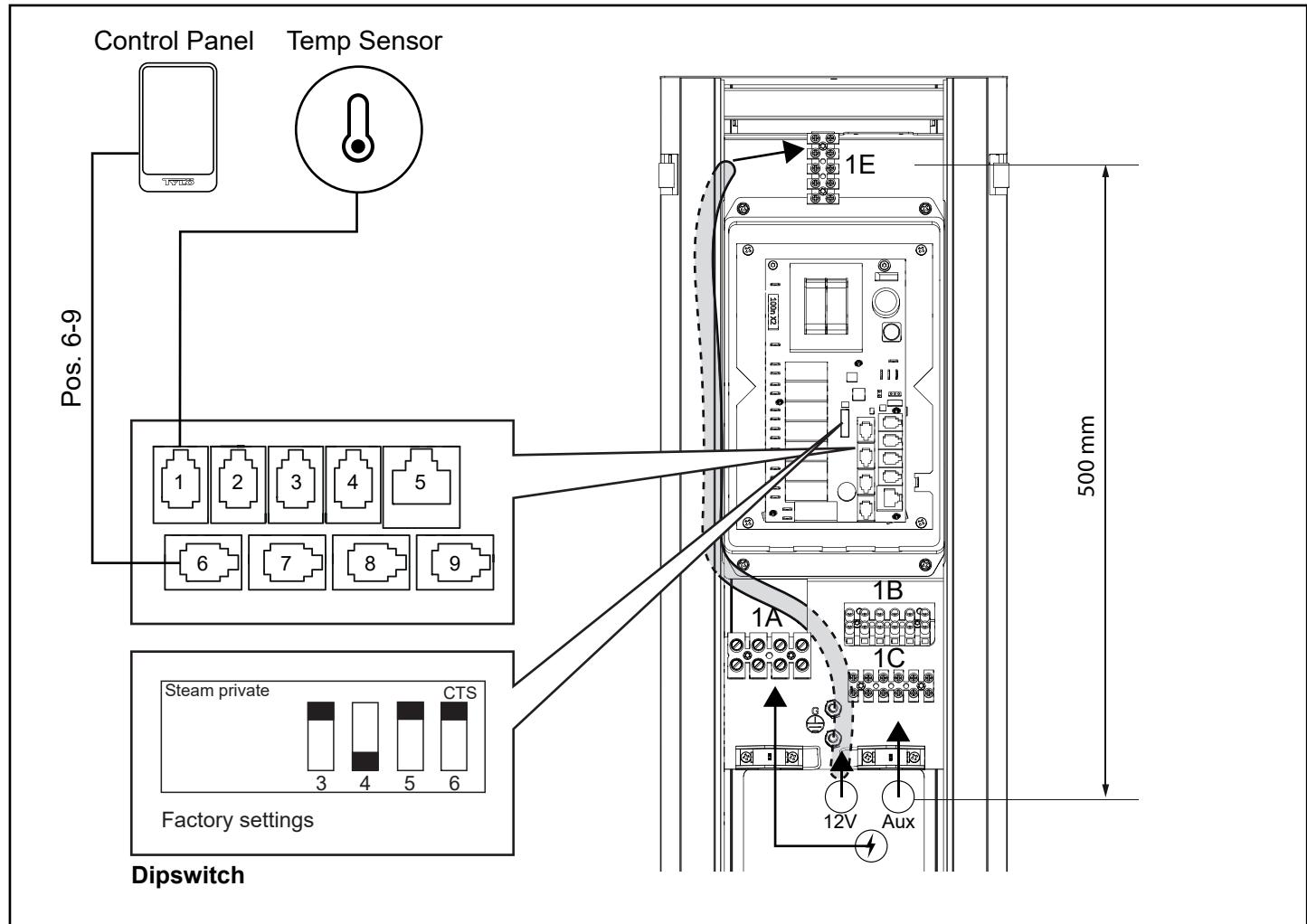
Fig.5 Schematic diagram of installation, Stella steam generator
