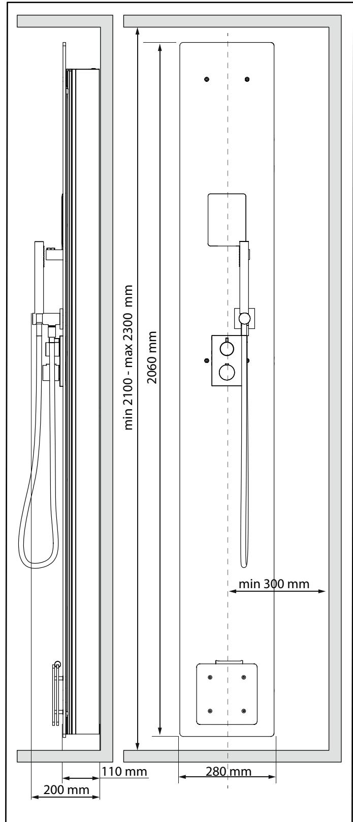
Fig. 1 Dimensions in millimetres, Steam column Stella type
