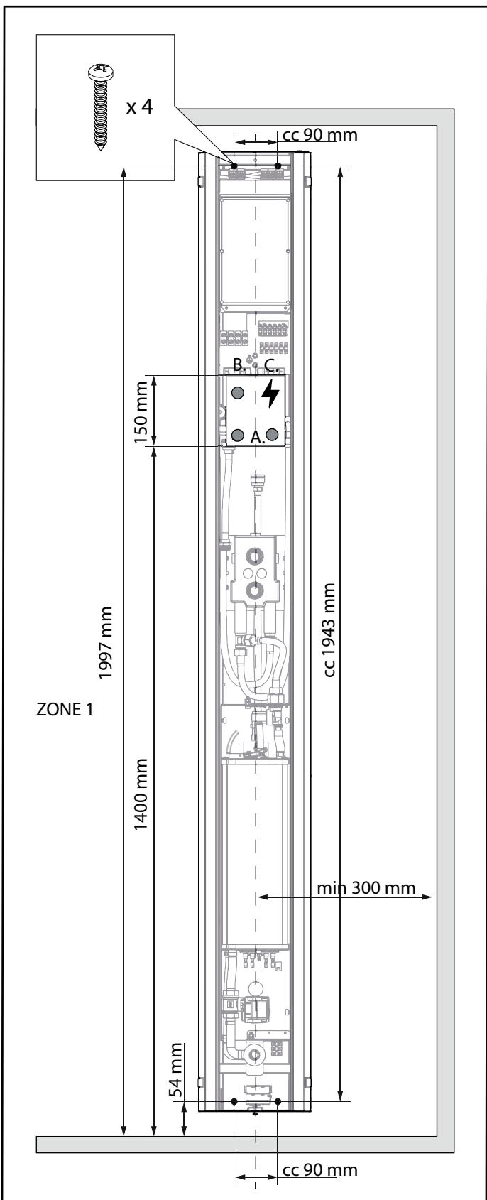
Fig. 2 Dimensions for installation, water and electrical connection
