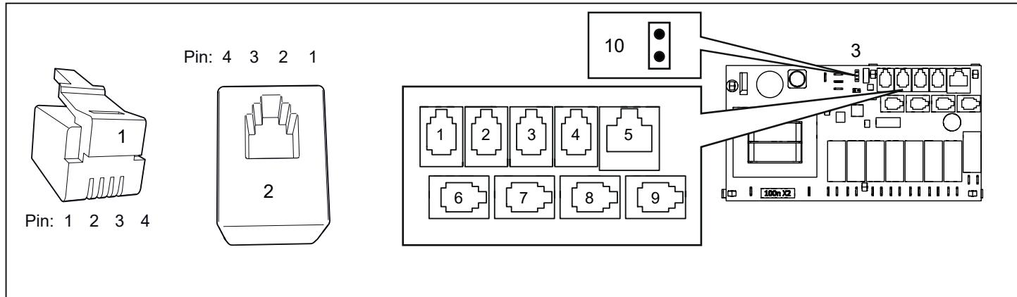
Fig. 10 Modular plug/modular contactor and relay board "high"
