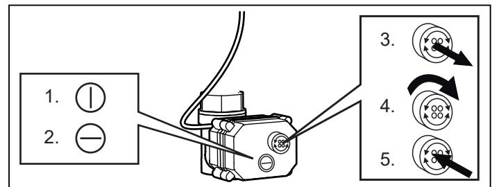
**Figure 18:** 1. Vertical line indicates open valve
